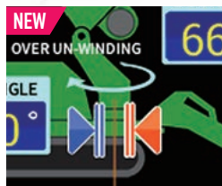
Working Range Setting for Slew Restriction
