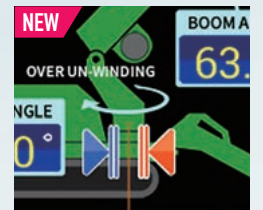
Working Range Setting for Slew Restriction
